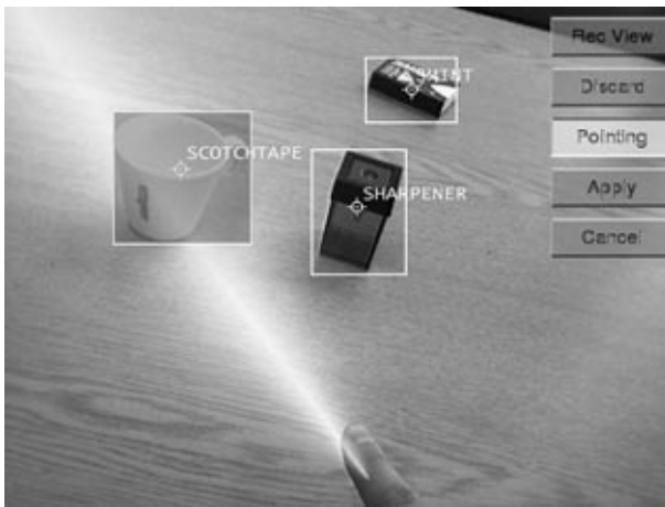
Fig. 2. User interface for interactive online learning. The user is pointing at a falsely classified object, which is highlighted as a feedback. To the right, virtual menu buttons are being displayed.
